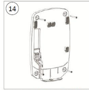
Screw the Plug-in base to the wall(x4)
