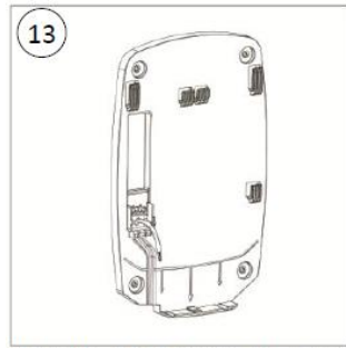
Route the wires through the Plug-in base as shown on the picture
