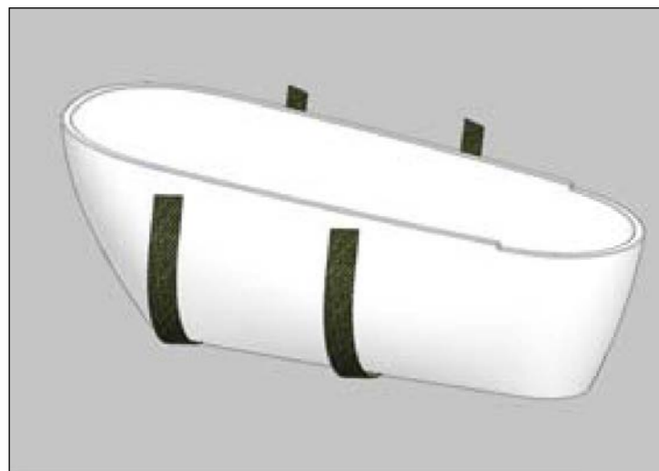
07 - Sollevare la vasca con due fasce come in figura. 07 - Lift the wash with two bends as shown in the picture.
