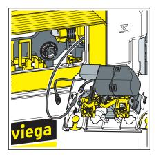
Create the plug connection from power pack to control.
