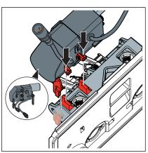
■ Place the control on the rear of the cover plate.
