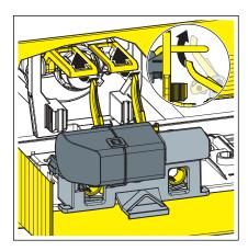
■ Hang the mechanism in the tab of the drain valve.
