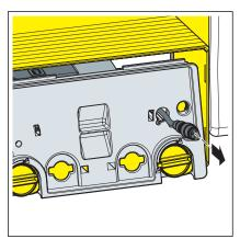
Guide the control cable forward through the right-hand opening of the front cover plate.
