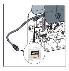
Apply the silicon grease to all connections of the control.
