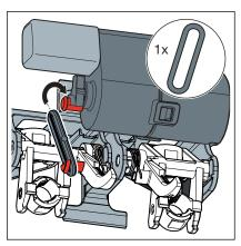
Connect the bow of the mechanism and the control with the eye.
