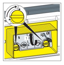
Turn the cover plate lock by 90° in a clockwise direction.
