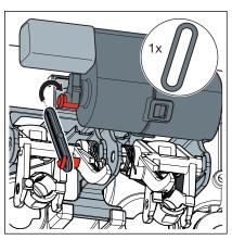
Connect the bow of the mechanism and the control with the eye.
